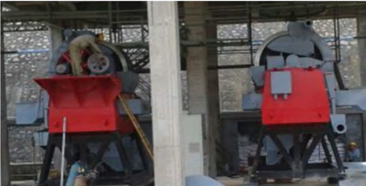
广东英德石英除铁 Iron removal of quartz in Yingde
