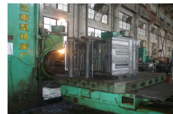
下铁芯加工 Making of the lower iron core
