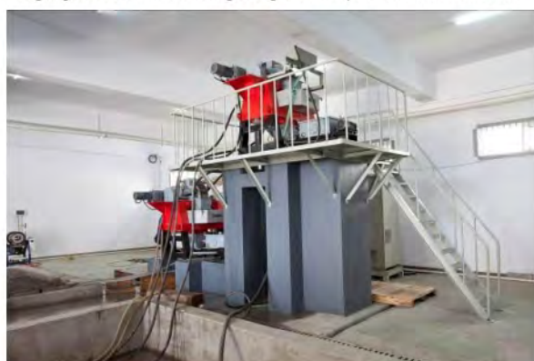
2级立环脉动高梯度磁选机 High gradient vertical ring magnetic separator with 2 levels
